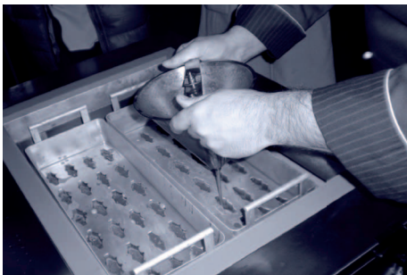
1. Fill the molds with the mix, using a dosing funnel.
